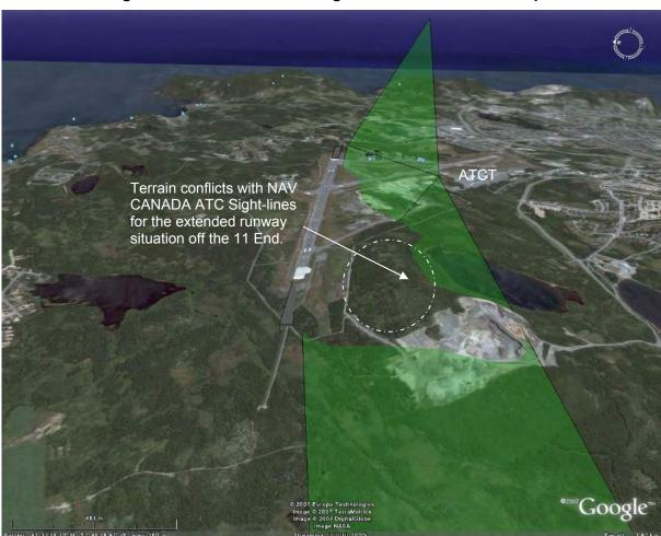
Figure 5-10 11 End ATCT Sight-Line Constraints – Proposed
