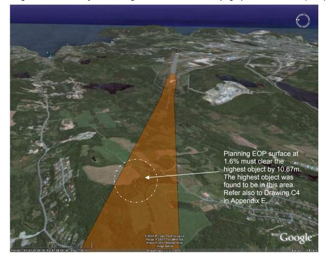
Figure 5-5 Runway 11 End Engine Out Performance Topographical Constraint (1.6%)
